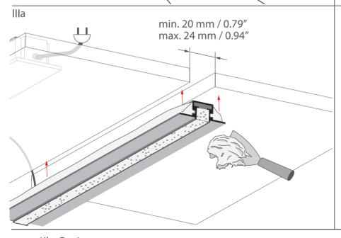
Place mounting adhesive on the backside of the flanges of the extrusion as shown in the drawing.
