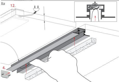
Lead the wire from the power supply (12) through the pre-drilled hole. Put the short end section of the cable into the groove inside the extrusion and put the insert back.
