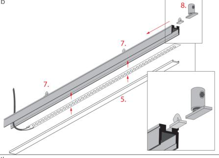
Insert the TEKNIK clips (7), and the FI-10-W fastener (8) into the outer groove of the extrusion. (small lock)
