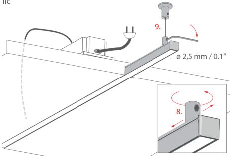
Lock the FI-10-W fastener (8) in the designated position, by screwing its head to the extrusion.
