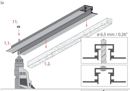
Remove protective insert (1.2) form TEPIKO extrusion (1.1).
