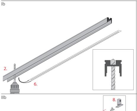
Drill the hole in the PIKO-ZM extrusion (2) along the same axis as the hole in the TEPIKO mounting track.
